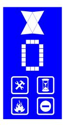
This display shows upper menu of Floor 0 (bottom floor). To edit Floor 0 display data, push ENT shortly and enter sub-menu.
