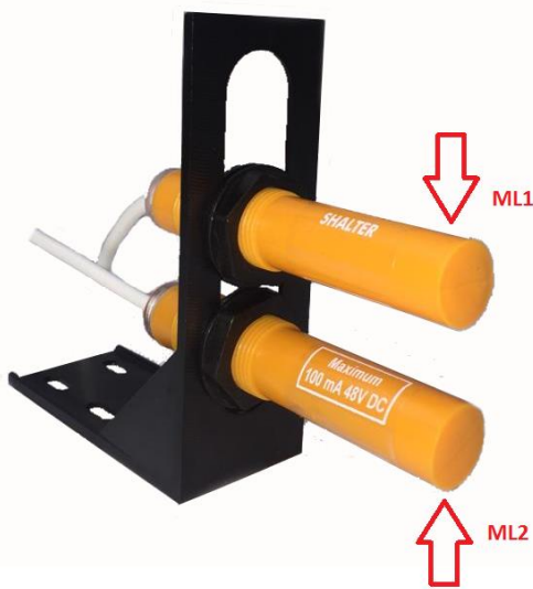
Figure 9- ML Magnet Position on Rail
