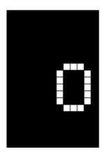
Here right char blinks. Now it can be changed by pushing INC ( $\uparrow$ ) and DEC ( $\downarrow$ ) buttons. Any number or letter can be chosen. After selecting right char, push ENT shortly and left char starts to blink. In the same way left char is set. Then select floor and signal color by pushing ENT and change with INC ( $\uparrow$ ) and DEC ( $\downarrow$ ) buttons. If no color selected to signals, then floor color displays.
