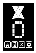
This display shows upper menu of Floor 0 (bottom floor). To edit Floor 0 display data, push ENT shortly and enter sub-menu.
