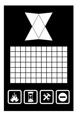
After initialization, software version number and ID (in CLC) is displayed first. Then inputs are evaluated and related character(s) are displayed according to stored settings. If no input is connected or all connected inputs are passive then stop 0 character(s) are displayed. (In 7-Segment Mode if no input is connected or connection is wrong then no character displays; if no communication established in CANBus mode, then "CE" displays)
